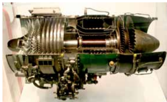
Cross section of a turbojet engine (ca. 1970).
